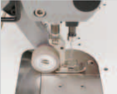
Puller with standard presser foot (closed)
