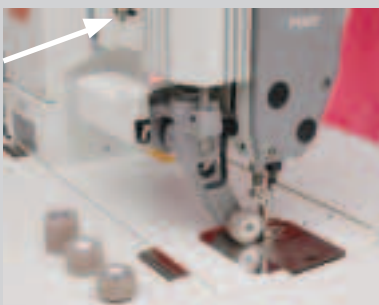
Easy adjustment to different puller widths
