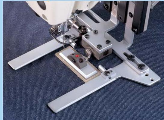
Sewing labels (FU05 type inverting clamp device)
