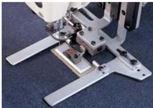
Pneumatic inverted clamp device
