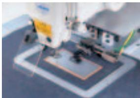
Pneumatic inverted clamp device
