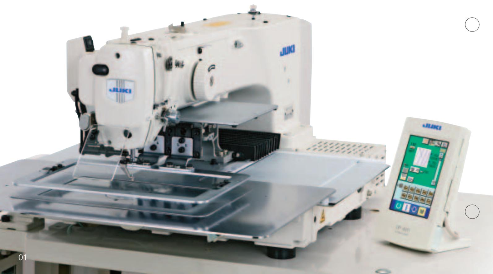
The machine has a wider sewing area and ensures the smooth placement of material. It supports improved seam quality with its highly-accurate sewing capabilities.
