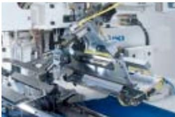
(\*The photo shows the automatic welting patch feeder with the welting patch cutting device installed.)
