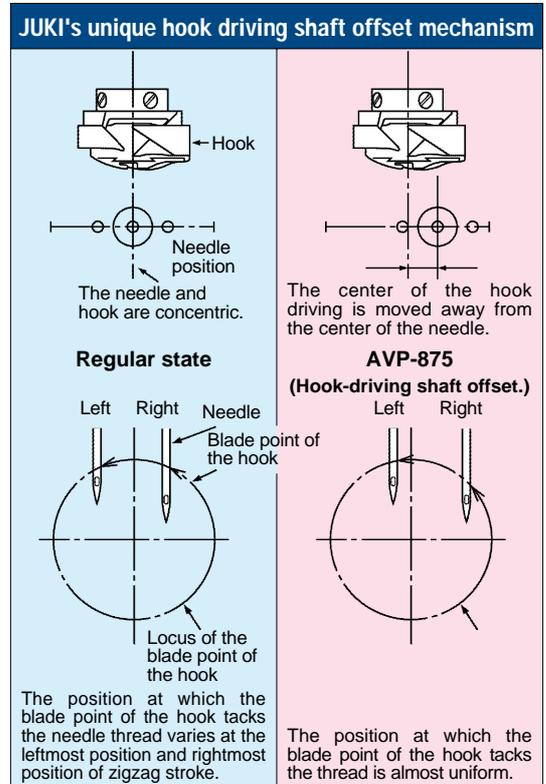
The blade point of the hook tucks the thread at a constant position even if the needle throws to the right and left, thereby helping reduce stitch skipping and thread breakage.
