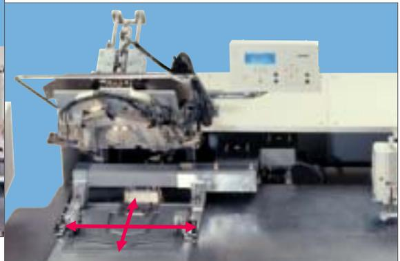
After replacing the pocket style jig, the folding position of the pocket cloth can be finely adjusted via the operation panel in a few short moments.
