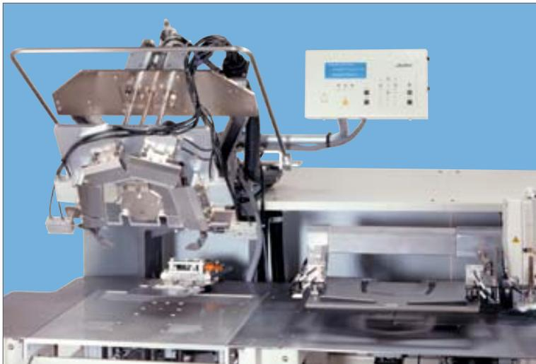
Pocket style jigs can be replaced with no tools. A new pocket style jig can be installed in the machine and fully adjusted in only about five minutes.
