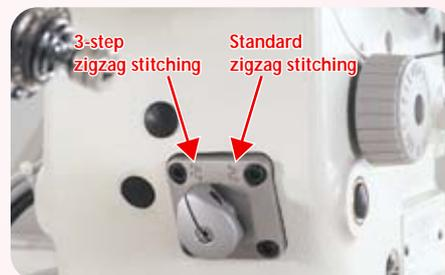
Standard/3-step zigzag stitching pattern changeover lever
