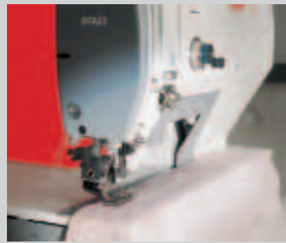
Off-set arm for easy placing/handling of workpiece
